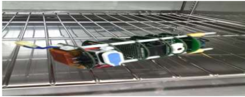
Fig. 4. Assembled structure, ready for starting a vacuum thermal cycle
