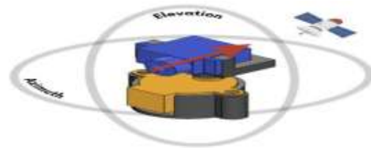
Figure 10. Rendering of Stepper and Servo motors being used as Azimuth and Elevation axes respectively.
