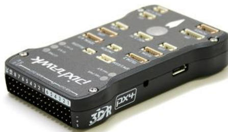
Figure (6) Pixhawk Board
