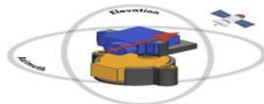
Figure 10. Rendering of Stepper and Servo motors being used as Azimuth and Elevation axes respectively.
